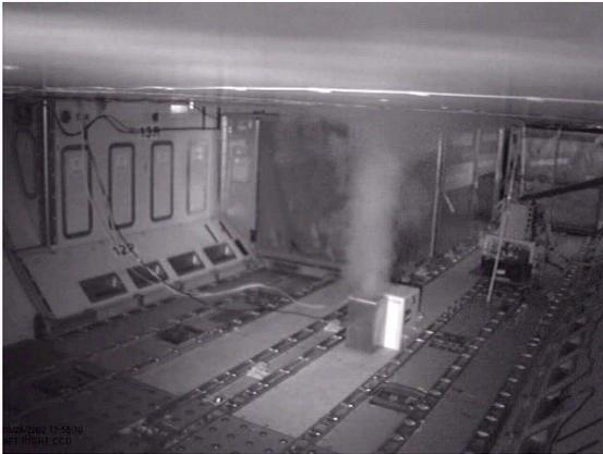
Fig. 4 Smoke generator test in A340-600 aircraft
