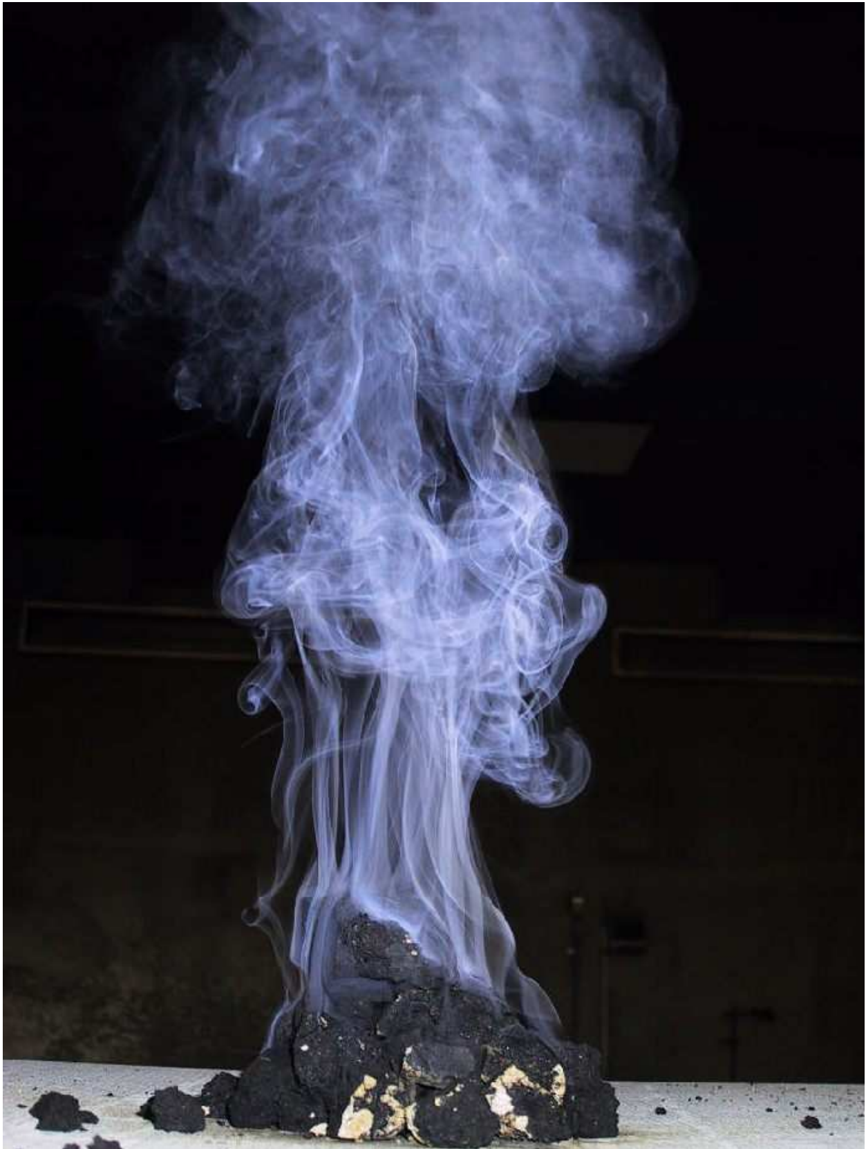
Smoldering coal fire for testing fire detectors
