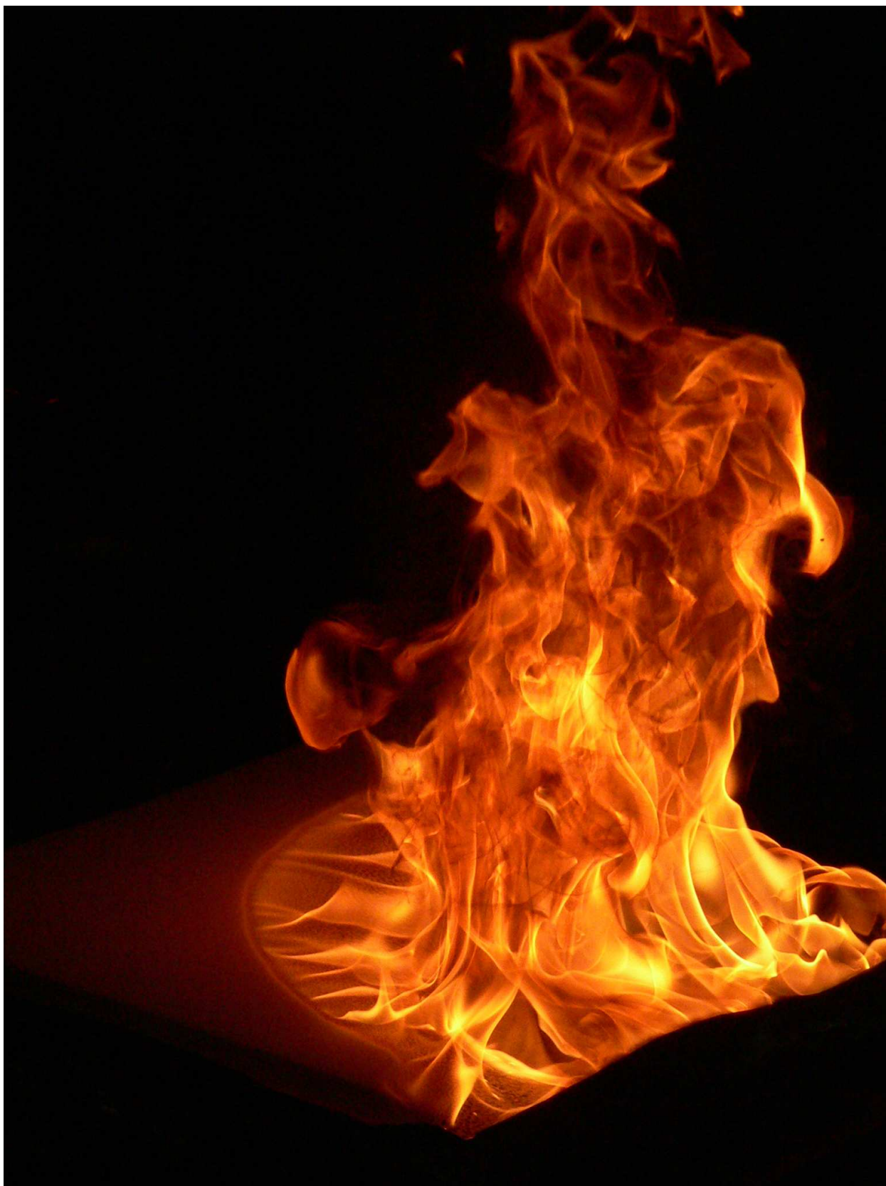
Flaming plastics fire TF 4 (polyurethane) defined by the European Standard EN 54 part 7 for testing fire detectors
