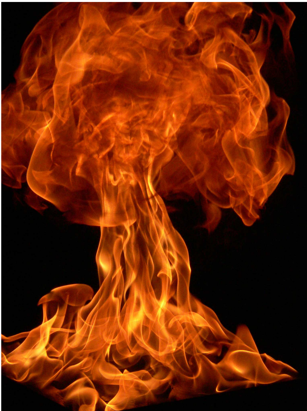
Flaming liquid fire TF 5 (n-heptane) defined by the European Standard EN 54 part 7 for testing fire detectors
